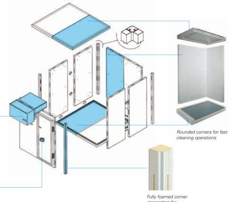
Fully foamed corner connection for optimal insulation
